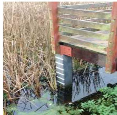
*Fig 4.4. Graduations on the base of the platform allow for easy measurement of the lake water levels.*
