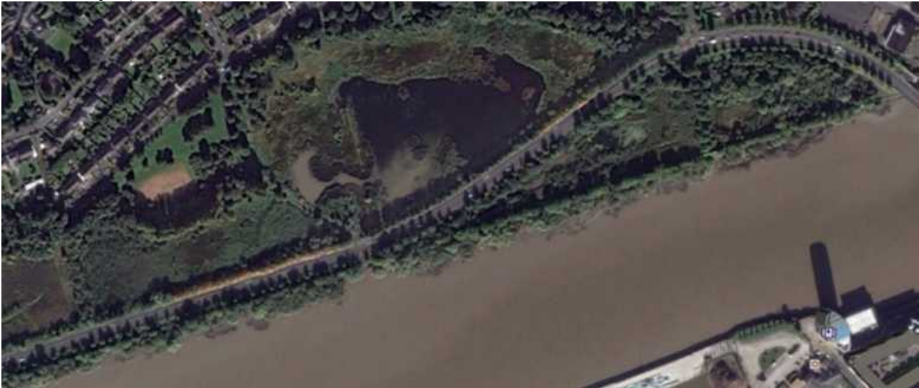
Figure A3.26. Suspended solids inflow during high tide (most likely following heavy rainfall).
